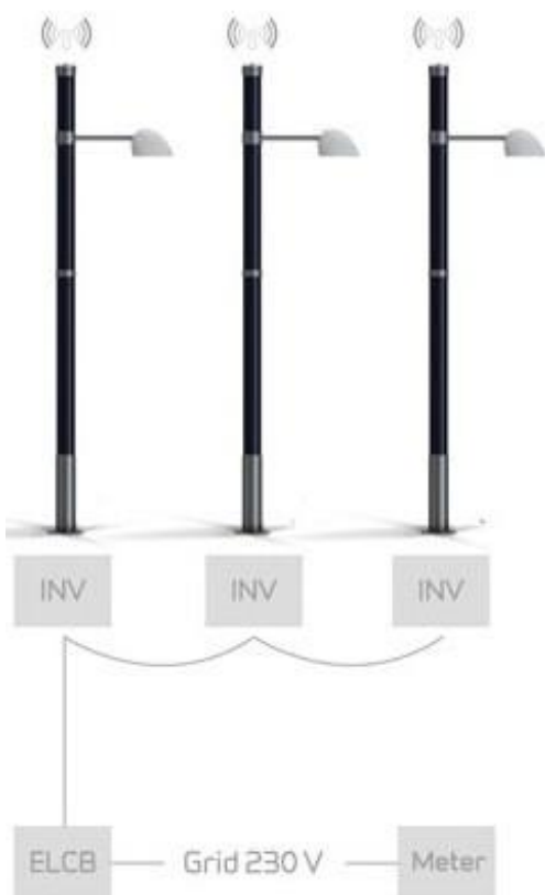
Communication (Zigbee between columns up to 400 metres)
