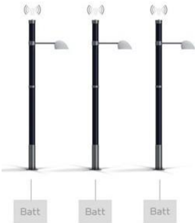
Communication (Zigbee between columns up to 400 metres)
